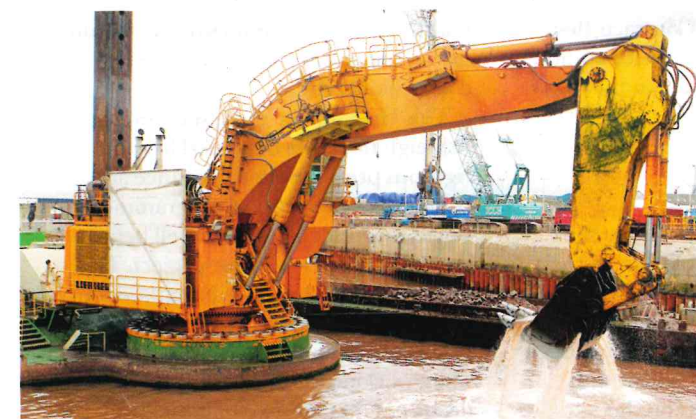
Above, below and below right: Boskalis used its MP40 backhoe dredger, the upper-structure of a 390-tonne Liebherr P995 mining excavator mounted on a spud-leg pontoon that measures 60m x 18m.
